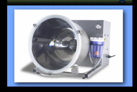
Tumbles proteins and liquids (such as brines and marinades) together under vacuum. The combination of low atmospheric pressure (caused by the vacuum) and the tumbling process, can reduce brine durations from hours and days to minutes.
